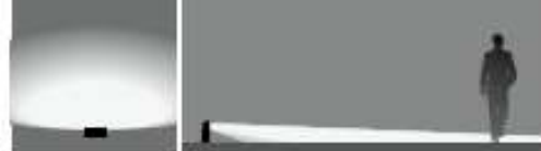
Asymmetrical flat beam light distribution
