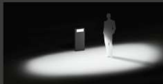
Asymmetrical flat beam light distribution
