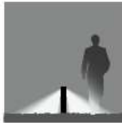
Height 600 mm: Symmetrical light distribution
